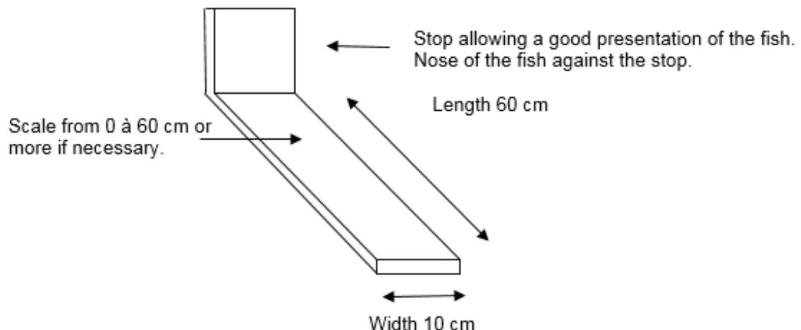
When a fish reaches the minimum size (12 cm in the Mediterranean resp. 18 cm in other seas) the fish is valid. In the case of the measurement system, the centimeters to be allocated must be rounded up, i.e. to 13 cm. This also applies to all subsequent measurements.
